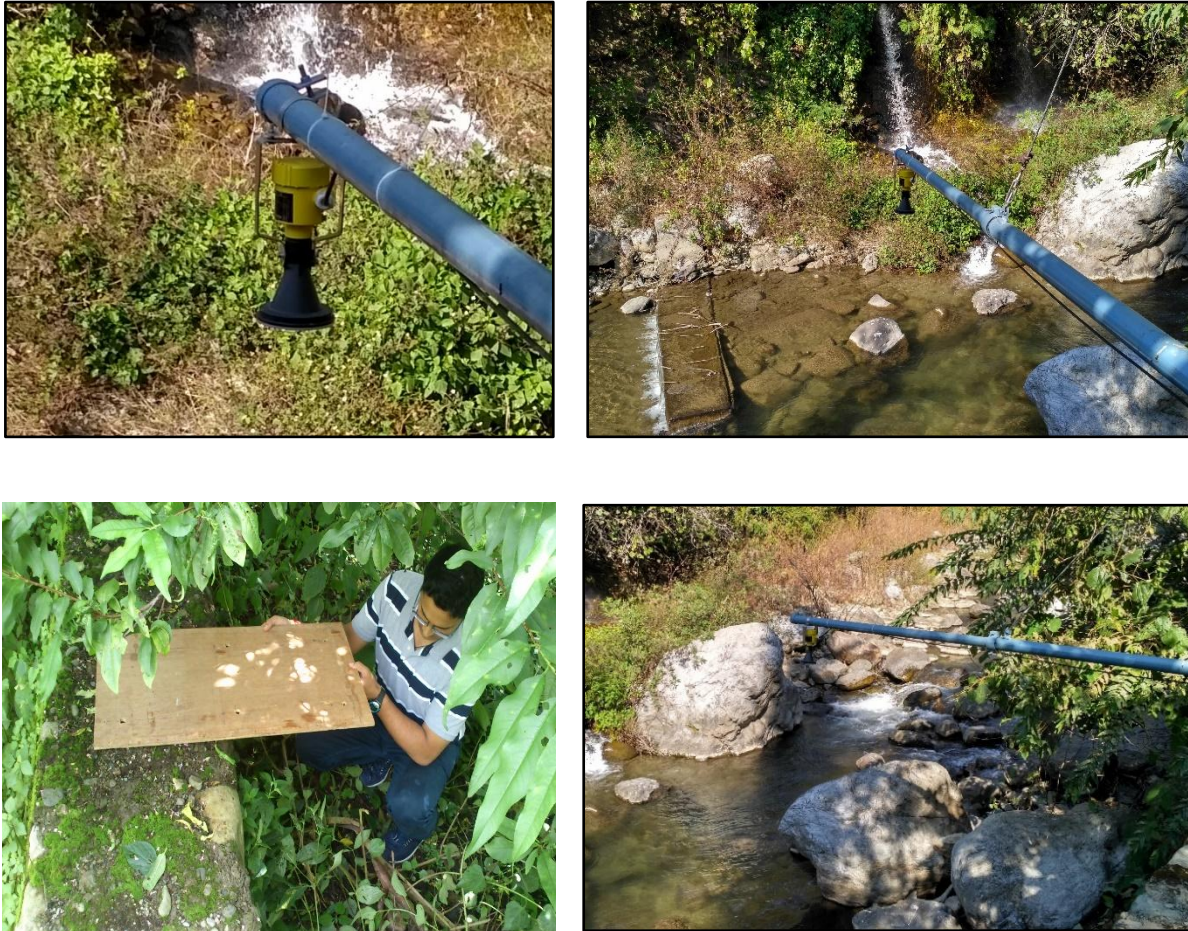
Fig. 3. 4: The digital water level recorder (DWLR) installed on the outlet of Henval stream
